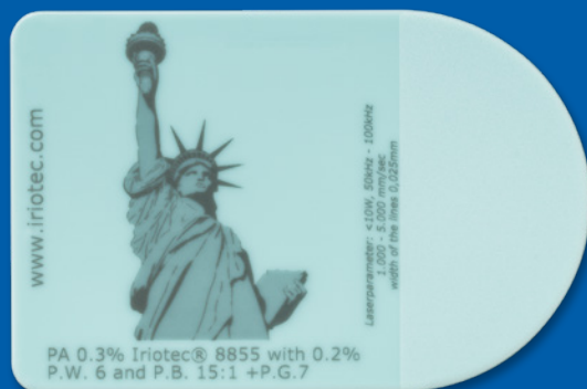
LASER MARKED PA CHIP WITH IRIOTEC® 8855
