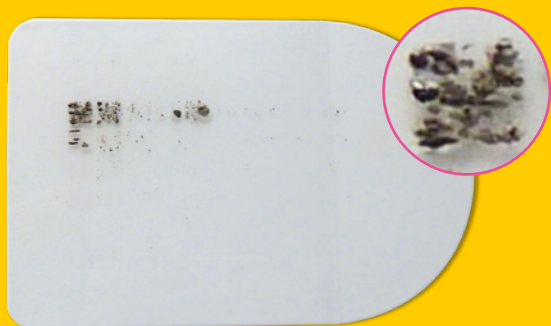
Test grid 500 – 5000 mm/s and 20 – 100 kHz
