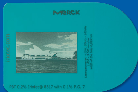
LASER MARKED PBT CHIP WITH IRIOTEC® 8817
