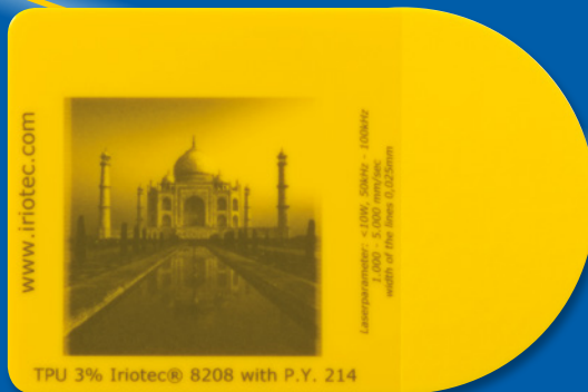
LASER MARKED YELLOW TPU CHIP WITH IRIOTEC® 8208
